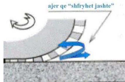
Fig 4.6 Efekti Air pumping [11]
