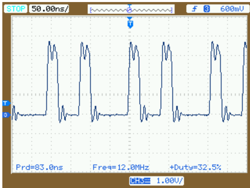
Fig. 8.4: Matja e frekuencës (Assembler)
