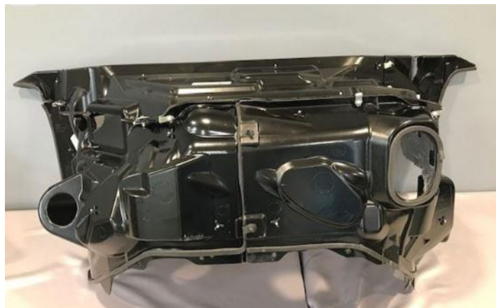
Figura 5.7. Muri dyanësor i motorit (Dual wall dash) i Ford Explorer 2020 [20]
