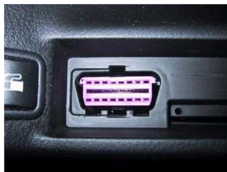
Figura 3.20: Kyçësi diagnostik sipas OBD II
